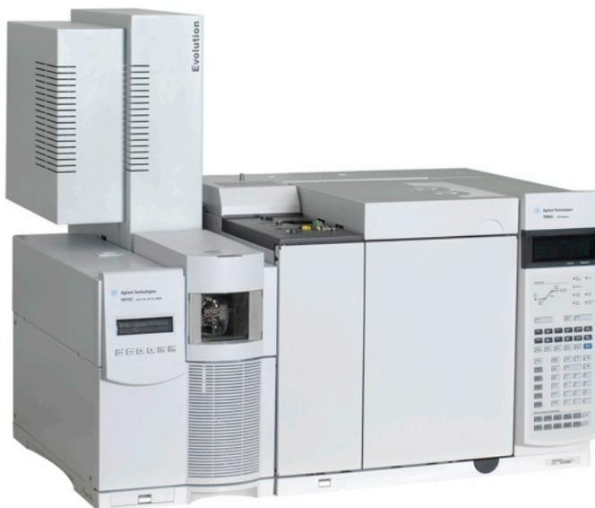
**Triple Quadrupole GC-MS/MS System**
